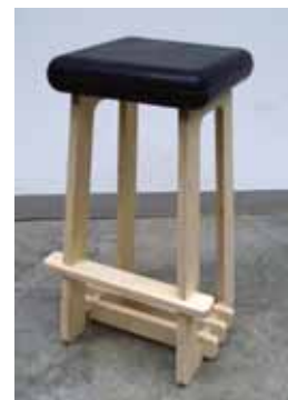
Figure 11: Rubber Stool by Steven Mullenbach; Stool modeled as "built" in form•Z, including all joinery, then CNC cut on the Techno router. The cushion was cast of urethane rubber in a mold modeled in Z and machined on the router.
