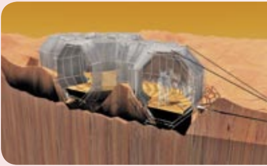
FIGURE 3: EARLY CUTAWAY SKETCH OF FACETED MODEL SET INTO REGOLITH. SOA/SABRE
