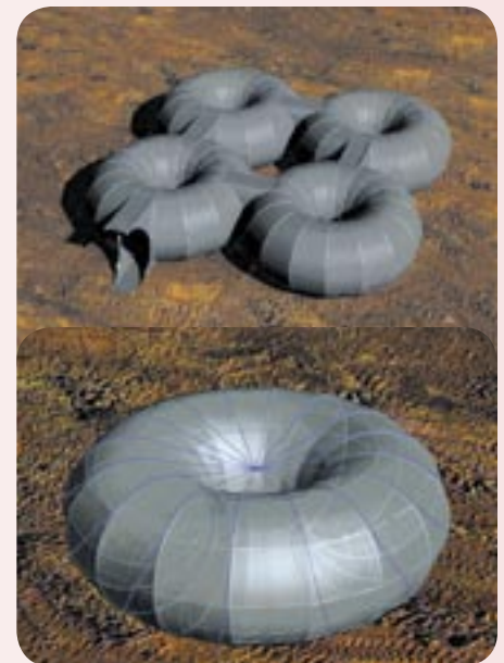
FIGURE 10: VIEW OF JOINED GRUB GREENHOUSES, LIVING MODULE OR SPACECRAFT REMOVED FOR SIMPLICITY AND DETAIL OF CONNECTOR SLEEVE.
