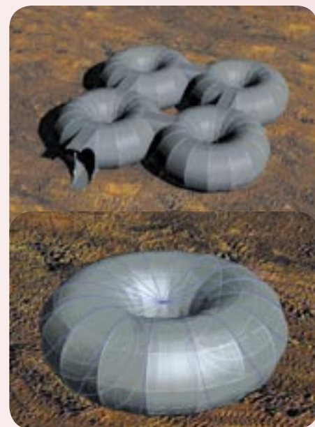
FIGURE 10: VIEW OF JOINED GRUB GREENHOUSES, LIVING MODULE OR SPACECRAFT REMOVED FOR SIMPLICITY AND DETAIL OF CONNECTOR SLEEVE.
