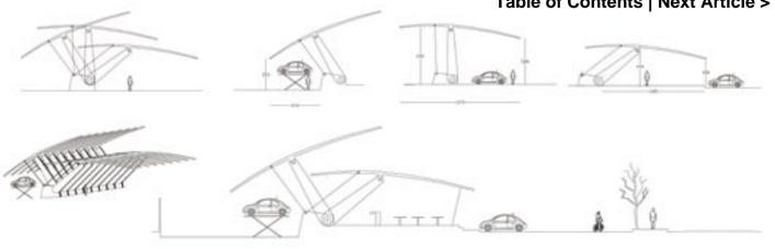
The module was designed as a Kit of metallic elements that can be made with laser cutting systems and CNC machines. Each module works by itself as a system of columns, tensions, and counterbalances. Several modules can be individually set or grouped in order to generate larger size publicity advertising that can be sold as an additional service offered by the module.
