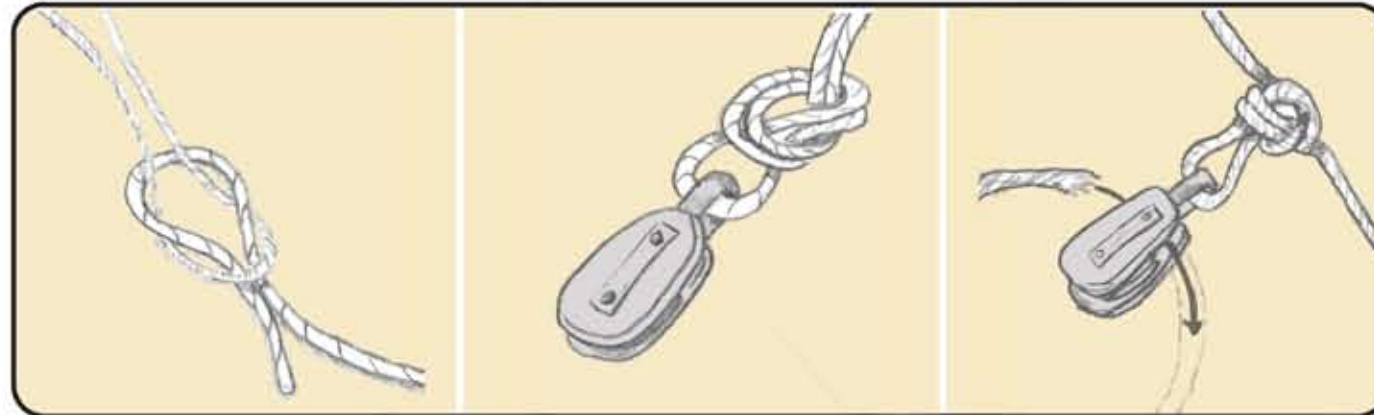
3. ATTACH OPPOSITE END OF LEADER TO NYLON ROPE. ATTACH PULLEY AT DESIRED HEIGHT ON NYLON ROPE.
